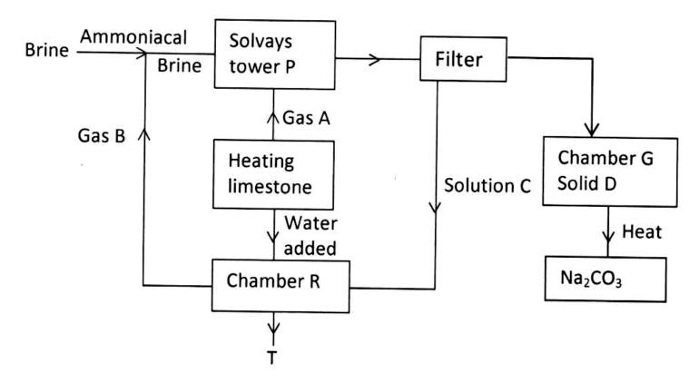
(a) Name gases A and B. (2mks) A – Carbon (IV) oxide $\sqrt{1}$
