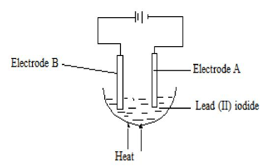
a) Why is heating necessary? (1mk) To melt the lead (II) iodide and form free ions (1mk)
